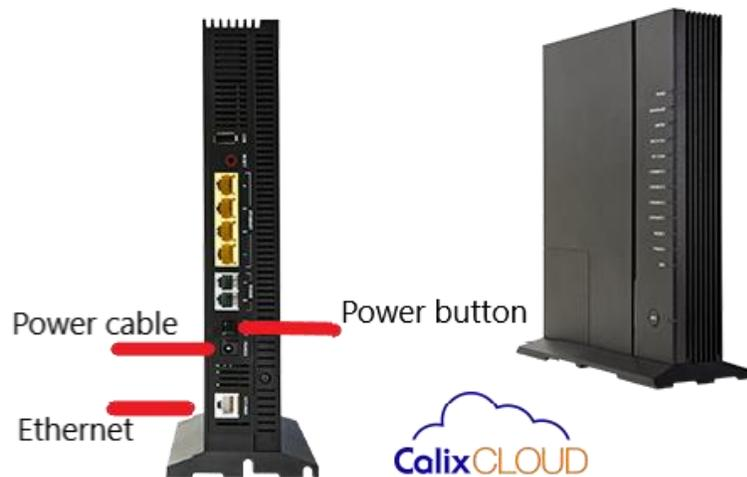
Step 4 – Once power and ethernet have been established, wait approximately 10 minutes for the new Blink router to download the correct Wifi information. When completed, the Blink router should be producing 2 wireless networks that correspond to the customers last name followed by “\_2.4” and “\_5ghz”. The password will always be set to the word blink followed by the customer number which is part of the customer’s account number with Barbourville Utilities.
